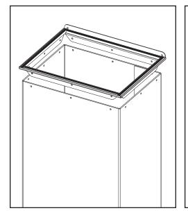
**4.** Insert the frame into the corrugated insert making sure the holes line up with the holes in the frame.
