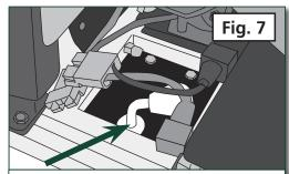
Attach the front Engine Clamp Knob
