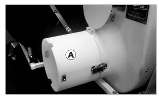
This is the Z-10 Extender Collar (A). It adds about 8 inches to the length of your mower deck hose to provide additional clearance around the rear wheel of your mower.
