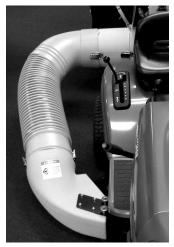
**3.** After the assembly is complete, there should be enough clearance so the rear wheel does not interfere with the deck hose.
