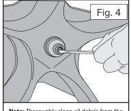
**Note:** Thoroughly clean all debris from the impeller bolt hex socket before trying to remove the bolt.
