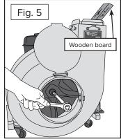
**TIP:** Because the engine frame is on wheels, it is helpful to clamp one or two short lengths of 2x4 to your work bench so the frame does not roll around. This is especially helpful if you are doing a one-person job.
