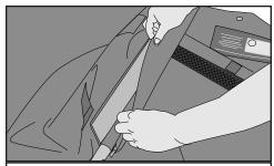
inserted, remove the plugs and secure the upper zipper or Velcro flap. Note: The Velcro strap should completely cover the Velcro strip on the collector bag.
