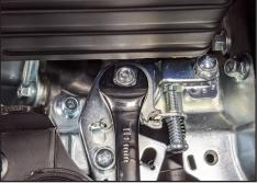
**4.** Use a 10mm open end wrench to tighten the nut in small increments.
