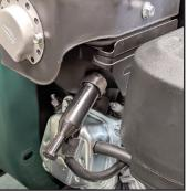
**1.** Locate the spark plug underneath the muffler. Pull the spark plug boot to disconnect.
