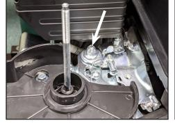
**3.** Locate the nylon-insert locknut at the pivot of the throttle lever.
