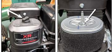
2. Locate the knob on top of the air filter cover, and remove the knob and cover. Then, remove the wingnut holding the air filter down and slide off the air filter.
