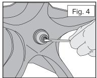
Note: Thoroughly clean all debris from the impeller bolt hex socket before trying to remove the bolt.
