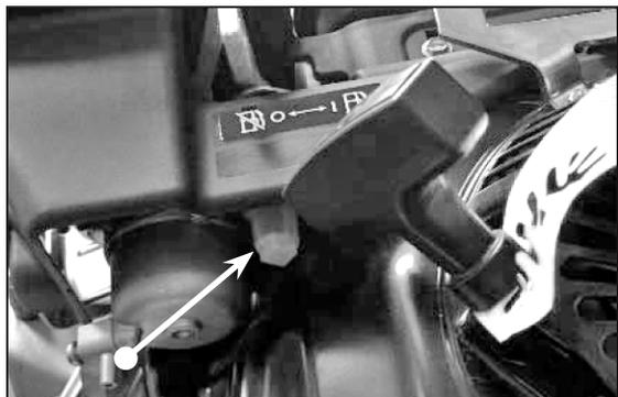
For 8 and 10 HP Vanguard engines, fuel bowl is beneath the red lever and somewhat hidden by the plastic shroud.
