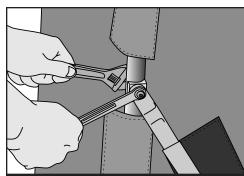
**3.** With the side link locked in place, disconnect the pivot bolt and lower the side link out of the way.
