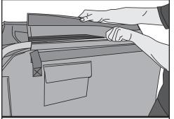
**2.** Open the Velcro strip, or top zipper that secures your collector bag to the top of the side tube.
