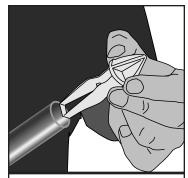
**8.** Place the plastic side tube insertion plugs into both ends of the new aluminum side tube.
