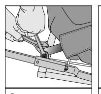
**4.** Disconnect the front and rear hinge bolts from the ends of the aluminum side tube.
