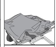
To Install the new side tube, start with the collector bag flat on the collector frame.
