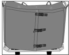
**3.** This shows the proper final adjustment. With the Velcro lined up, the buckles will snap together without excess slack or excess tension on the webbing.
