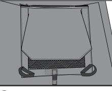
**2.** When properly aligned, no Velcro should be visible around the top screen, and the rear Velcro strap will be in place to hold the top screen.
