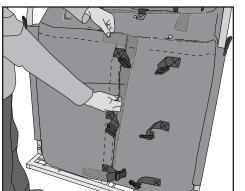
**1.** Close the three inner buckles. Then carefully close the outer doors so the Velcro strips overlap. *Note: for new collector bags, the fabric may be stiff and this adjustment may require some pulling. The fabric will relax with use.*
