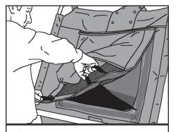
**1**. Raise the collector frame and lock it in the dump position. Lift the top screen as shown to release the Velcro on all 3 sides. Then carefully lower the screen to align the Velcro on one side. Run your hands along all three sides to press the Velcro together.
