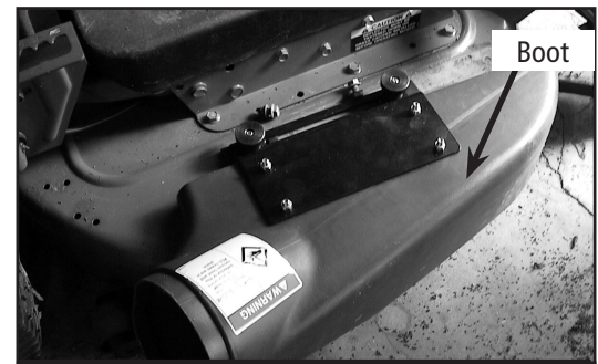
Finished assembly of the V Mower Deck Adapter™ with quick release deck connection.
