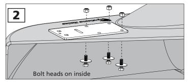
3. Install the three 5/16 x 1-inch bolts, each with a 5/16 fender washer, up through the inside of the boot and the boot plate. Secure with the 5/16 nylon lock nuts. (Fig. 2)
