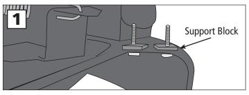
2. Push the two 1.5-inch bolts up through the bottom of the mower deck and screw them into the threaded holes in the small rectangular Support Blocks. Tighten firmly with a wrench. You will now have two threaded studs protruding from your mower deck. (Fig. 1)
