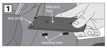
Remove the hinged grass deflector shield and hinge bracket from your mower deck to expose the deck opening and the two mounting holes. Connect the mower deck spring to the M46-Deck Plate as shown and place the Deck Plate over the holes in the mower deck.
