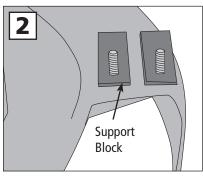
2. Push the two 1.5-inch bolts up through the bottom of the mower deck and screw them into the threaded holes in the small rectangular Support Blocks. Tighten firmly with a wrench. You will now have two threaded studs protruding from your mower deck.
