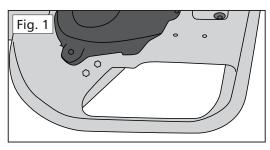
1. Remove the hinged grass deflector from your mower deck to expose the deck opening (Fig. 1). On most machines this is just a matter of removing two bolts.
