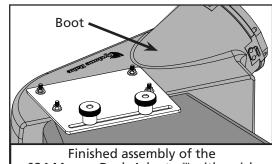
Finished assembly of the 024 Mower Deck Adapter™ with quick release deck connection.
