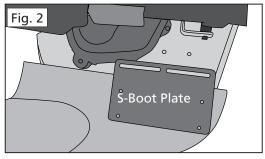
2. Hold the pre-cut boot up against the mower deck opening and place the S-Boot Plate on top of the boot. The slotted portion will hang over the top of the mower deck surface (Fig. 2).
