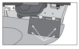
4. Position the boot under the boot plate and flush against the deck opening. While holding the boot in place, mark the four bolt hole positions with a marker pen (Fig 4). Loosen the Clamp Knobs and remove the Boot Plate from your mower deck.
