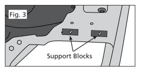
3. Trace the outline of the slots onto your mower deck with a marker pen. Drill two 5/16" holes for the mounting bolts within each slot range. Push the two 5/16" x 1.5" bolts up through the bottom of the mower deck and screw them into the threaded holes in the Support Blocks. You will now have two threaded studs protruding up from your mower deck (Fig 3). Drop the Boot Plate over the threaded studs and spin on the Boot Plate Clamp Knobs.
