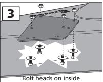
3. Install the boot plate with the four 5/16 x 1-inch bolts, each with a 5/16 fender washer, up through the inside of the boot and the boot plate. Secure with the 5/16 nylon lock nuts.
