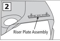
2. Attach the Riser Plate Assembly to the mower deck using two 5/16 x 1-inch bolts washers and lock nuts. Put the two 5/16 washers under the nuts.
