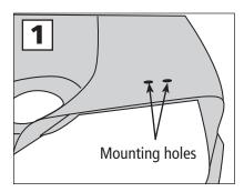
1. Remove the hinged grass deflector from your mower deck to expose the deck opening and the two mounting holes.
