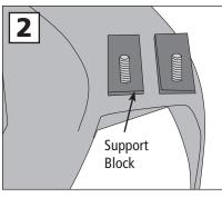
2. Push the two 1.5-inch bolts up through the bottom of the mower deck and screw them into the threaded holes in the small rectangular Support Blocks. Tighten firmly with a wrench. You will now have two threaded studs protruding from your mower deck.
