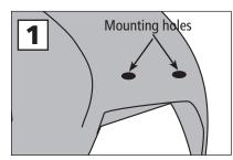
1. Remove the hinged grass deflector shield and hinge bracket from your mower deck to expose the deck opening and the two mounting holes.
