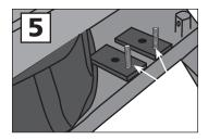
Push the two 5/16 x 1.5 inch bolts up through the bottom of the mower deck and screw them into the threaded holes in the support blocks. You will now have twotreaded studs protruding up from your deck.
