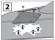
2. Install the four 5/16 x 1-inch bolts, each with a 5/16 fender washer, up through the inside of the boot and the boot plate. Secure with the 5/16 nylon lock nuts.
