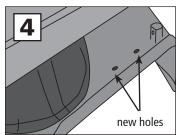
4. Drill the first hole. Start with the 1/4" drill bit, followed by the 5/16" bit. Use the boot plate as a guide when drilling the second hole, so your holes line up.
