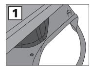
Remove the hinged grass deflector from your mower deck to expose the deck opening.
