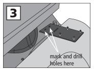
3. Position the MDA and Boot Plate over the opening in the mower deck. Mark the location of the first hole in the Boot Plate onto the mower deck.
