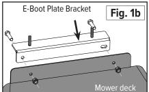
2. Position the E-Boot Plate Bracket over the existing holes in the mower deck flange. If the holes do not line-up, trace the outline of the holes onto the mower deck flange with a marker pen, then drill two 5/16" holes for the mounting bolts (Fig. 1a).
