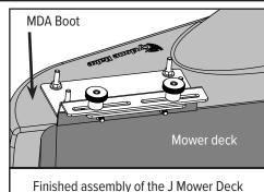
Finished assembly of the J Mower Deck Adapter with quick release deck connection.
