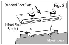
3. Bolt the E-Boot Plate Bracket to the mower deck using the two 5/16 bolts and nuts. Thread the two 5/16 x 1.5-inch full thread bolts up through the E-Boot Plate Bracket. Drop the Standard Boot Plate over the bolts and spin on the Boot Plate Clamp Knobs (Fig. 2).
