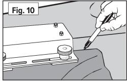
2. Hold the boot snugly against the lower surface of the plate directly in front of the deck opening (the boot may be moved forward or backward as necessary for installation). Mark the four bolt hole positions with the marker pen (Fig. 7). Loosen the clamp knobs and remove the boot plate from your mower deck.
