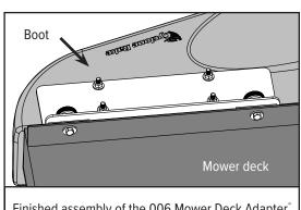
Finished assembly of the 006 Mower Deck Adapter with quick release deck connection
