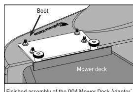
Finished assembly of the 004 Mower Deck Adapter with quick release deck connection.
