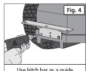
Use hitch bar as a guide when drilling second hole.
