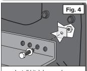
Install hitch bar washers inside mower
