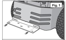
Standard hitch mowers have a flat metal plate between the rear wheels. The hitch bar bolts directly to the plate.
