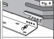
Install the reinforcement plate behind the mower plate.
